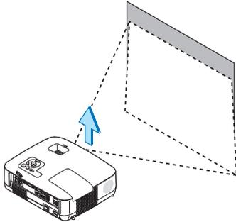
Adjusting the left and right tilt of an image
