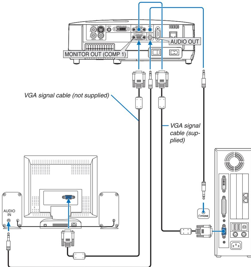
You can connect a separate, external monitor to your projector to simultaneously view on a monitor the computer analog image you're projecting.
