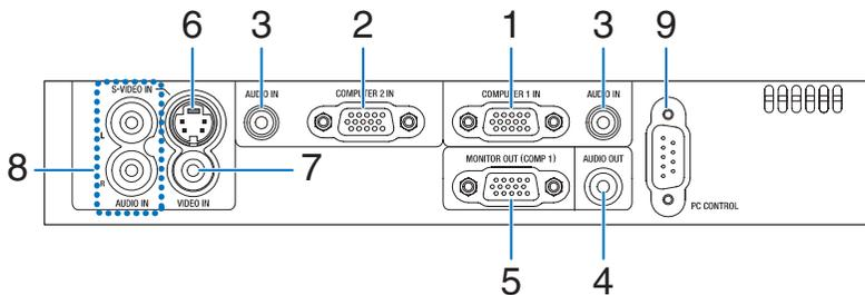
1. **COMPUTER 1 IN/ Component Input Connector (Mini D-Sub 15 Pin)** (→ page [17](#), [20](#), [22](#))
