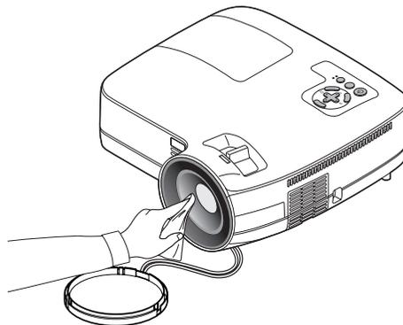
The NP610S and NP510WS have a plastic lens. Use a commercially available plastic lens cleaner.
