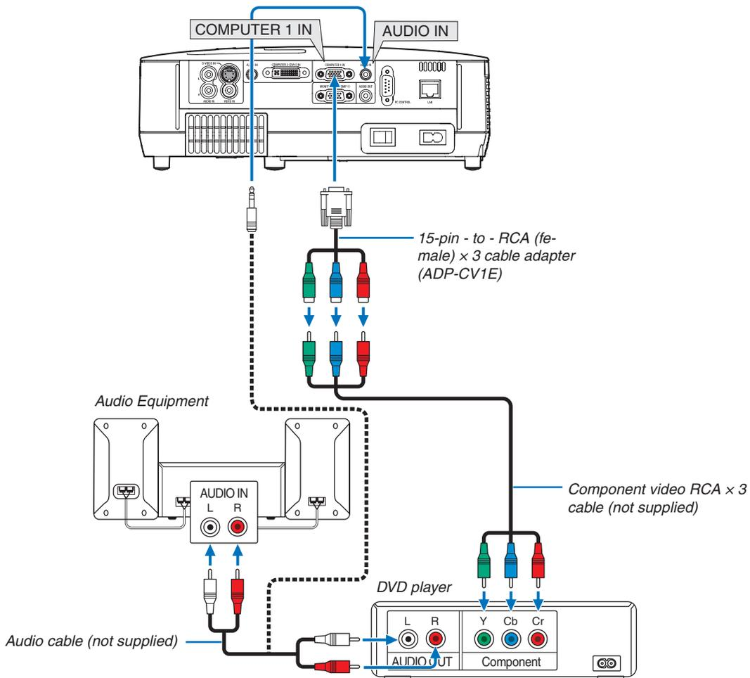
A component signal will be automatically displayed. If not, from the menu, select [SETUP] → [OPTIONS(1)] → [SIGNAL SELECT] → [COMPUTER1], and then place a check mark in the Component radio button.
