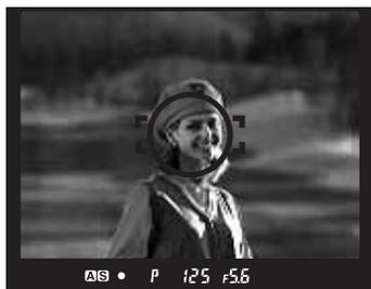
**[ ]** on the viewfinder LCL blinks to indicate the exposure is locked, when you continue to take the next picture in the AE lock mode.
