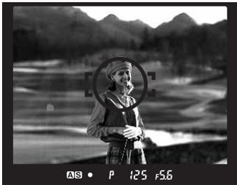
When the focus mark ● lights, the picture is in focus.
