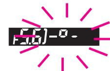
★ If the difference between the set value and the metered value exceeds 6EV, the viewfinder LCD blinks "– 0 –" for underexposure and "– 0 –" for overexposure.
