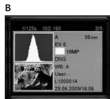
**B:** Most pixels are of medium brightness: Correct exposure
