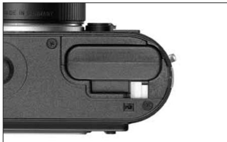
3. Inset the battery into the compartment with its contacts facing forwards. Press it into the compartment (1.37) until the white sprung locking catch (1.38) moves over the battery to hold it in place.
