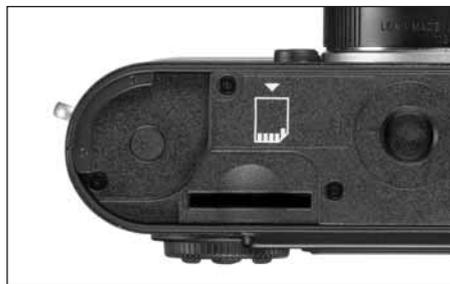
3. Insert the memory card into the slot (1.42) with the contacts at the back and with the beveled corner pointing downwards. Slide it completely into the slot against the spring resistance until you hear it click into place.
