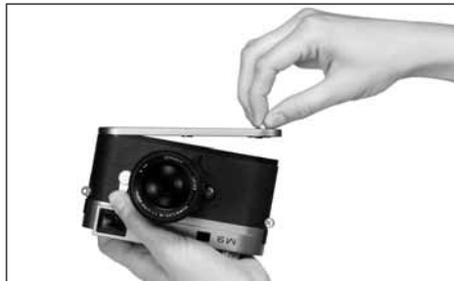
2. Remove the bottom cover (1.35) of the camera.
