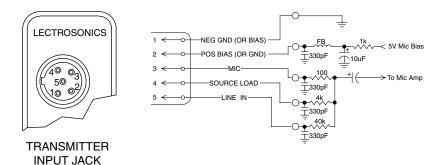
The best RF protection is accomplished by installing RF bypass capacitors at the mic capsule. If this is not possible, or if you are still having problems, capacitors can be installed on the mic pins inside the TA5F connector housing.
