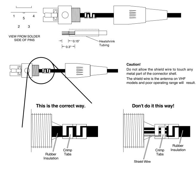
NOTE: This termination is required on VHF transmitters and will still work fine on UHF transmitters.
