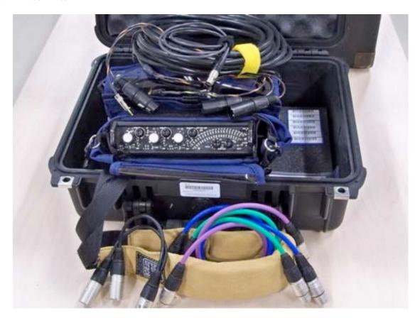
Sound Devices 302 is a 3 channel mixer with Mid-Side capabilities for stereo recording. The pouch has enough room for additional gear such as 3 wireless receivers. This kit is designed for supplying audio to a camera or several recording devices. There is a 20 ft. Breakout cable with two XLR's and return audio paths to monitor from other devices. The included XLR "Y" cable allows audio to feed (2) other devices at same time for a multi camera shoot. 3 AA batteries NOT INCLUDED.
