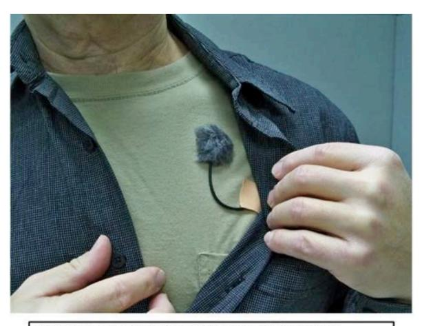
MICING WITH RYCOTE STICKY AND OVERCOVER. CLEANER AND FASTER. NOW WITH RYCOTE WINDJAMMER OVERCOVER ONTO STICKY.
