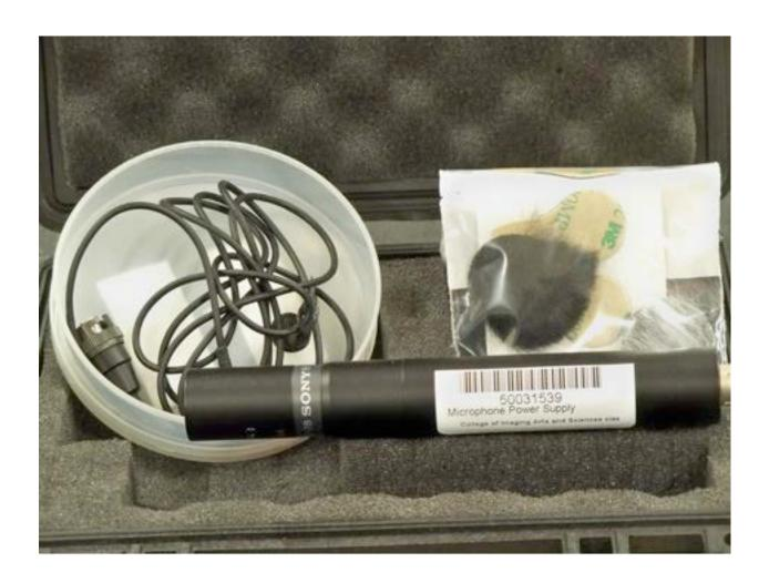
These kits are hardwired Sony ECM 77BC w/power supply (LDC-78). Included are Rycote over-covers and stickies. This mic can use 48V phantom OR internal AA battery "not included" Recommendations:
