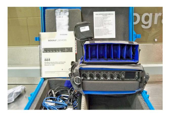
Sound devices 664 kit is a 6 channel mixer that can record and mix 6 microphones separately on discrete track. It can also record 12 individual tracks depending on the mode and menu settings. It also includes a break out cable to feed a camera and monitor audio from the camera and can generate and connect time code. This unit needs 5AA batteries and can use an SD or CF card (NONE INCLUDED). Auxiliary porta brace case for wireless mics
