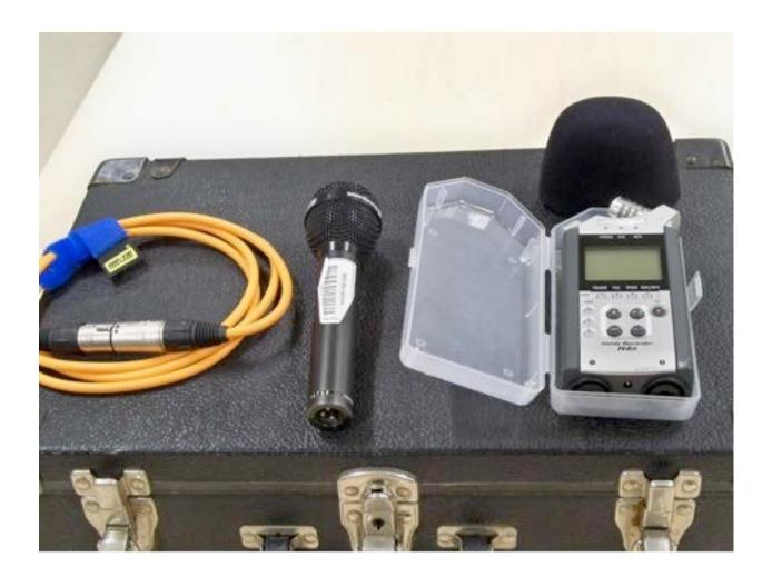
There are 6 of these kits each containing a Zoom H4n flash recorder with Beyer Dynamic cardioid M69 microphone and 1 10ft XLR cable. This recorder has an X-Y co-incident mic pattern for recording Stereo ambience. It also has two rear XLR combo jack inputs to record any type of microphone. It supplies 48V Phantom power and can do M-S matrixing but is recorded that way, no option for listening "only MS mode" such as 702 units can. 2 AA batteries
