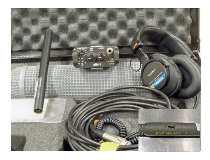
This kit contains a Sennheiser MKH 416T mono shotgun 12V T powered microphone. Included is Sound Devices MM-1 pre-amp that provides both 12v T & 48V phantom power. This kit includes other items; a Zeppelin windjammer with pistol grip, Headphones and a 25ft XLR cable. (Boom pole needed)
