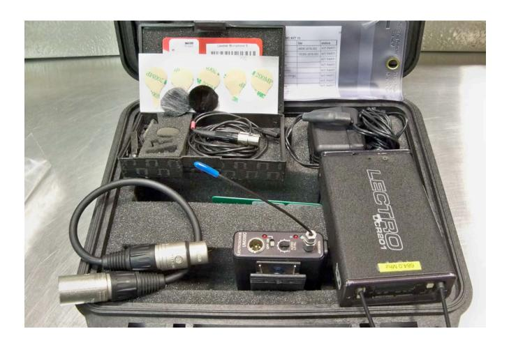
This kits contains a single pair of Lectrosonics UHF wireless transmitter – receiver combination with Tram "TR-50" Lav microphone. Please check written documentation for frequency choice (DO NOT CHANGE) and battery types (Not included).
