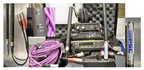
Mic pre-amp with stereo 5 pinY cord /two XLR's Black is both Mid capsule and left when stereo Red is both Side capsule and right when stereo Stereo mic switches: MS is 2 separate capsules. M is cardiod & S is figure 8 LR-W & LR-N is stereo already decoded Wide and Narrow
