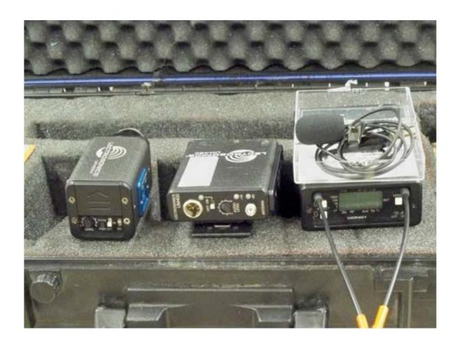
This kit contains and Lectrosonics UHF wireless receiver with 2 Transmitters. One is a "CUBE" for use on microphones and supplies 48v phantom power (not 12T power). The other is a transmitter (body pack style) with included Lectrosonics Lav microphone. WARNING: only one transmitter can be used or turned at a time! Please check written documentation for frequency choice and battery types (Not included).
