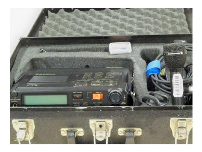
This kit contains a Marantz PMD 670 Compact Flash recorder with Beyer Dynamic cardioid M69 microphone and 1 10ft XLR cable. USB cable with Flash card reader included. This deck records 2 channels with mic and line inputs. It is industry standard for radio news reporters, specifically NPR and possibly BBC. Designed for back and forth interviews. It can use any type of microphone for other applications.
