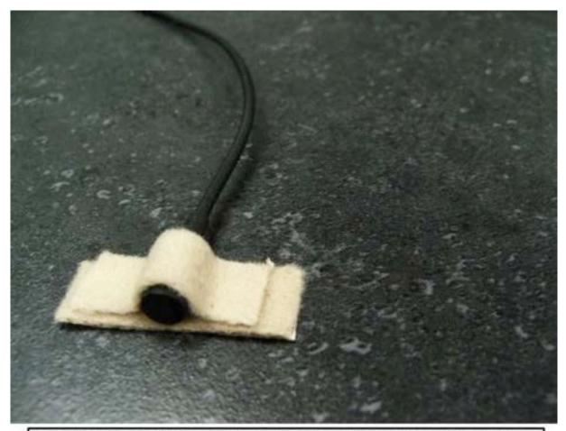
USING MOLESKIN TO PREPARE MIC FOR UNDER GARMET MICING TECHNIQUE. THE KEY IS TRYING TO AVOID MOVEMENT NOISE FROM CLOTHES. CUT STRIPS AND FASHION THIS WAY. IT WORLKS PRETTY WELL AND IS COST EFFECTIVE.
