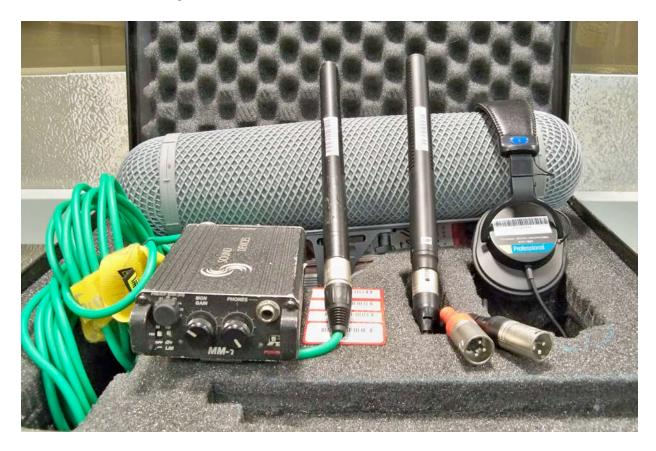
This kit contains Audio Technica BP4029 Stereo shotgun with adapter (5 pin XLR to (2) 3 pin XLRS). It also has a Sennheiser mono shotgun with an MM1 preamp which supplies and can only use 12v Tpower. Included are 2 (15ft) XLR cables, Headphones and Zeppelin windjammer and pistol grip.
